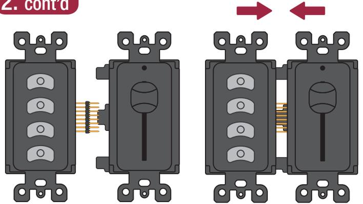
3. Verify proper contact by looking at the pins between the two inserts.
